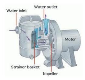
**How it Works:** Electric motor spins the impeller in the pump, which drives the water from the drain, through the filter, back to the pool through the returns
